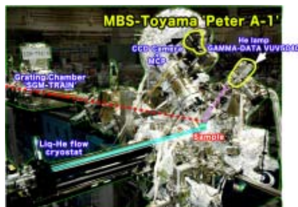
Fig. 2. High-resolution angle-resolved photoemission apparatus for BL5U
